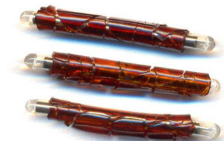
Figure 2: Thick acrylate coatings crack after heating to 250 °C when applied onto a glass rod due to differing thermal expansion coefficients. The magnet inside the glass rod is left with some expansion space for the same reason.
