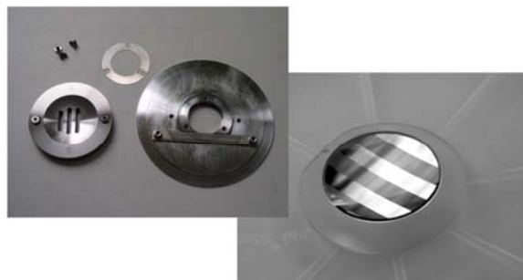
Figure 2: Etching mask (left), substrate holder (middle) and Al-coated master grating with two different blazed regions arranged in a stripe pattern (right).
